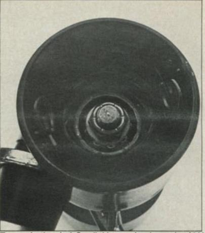
The open bearing wheel. So called because there is no seal or shield covering the balls. The balls are held against the "cup" inside the wheel by a "cone". This is held in position by a lock nut at the end of the axle.
