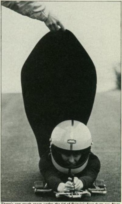
There's not much room under the lid of Britain's first skate car. Note the up-front vertical steering rod.
